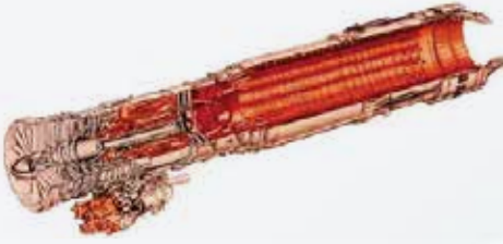
Figure 1. J85 Turbojet Engine with Afterburner [8]
