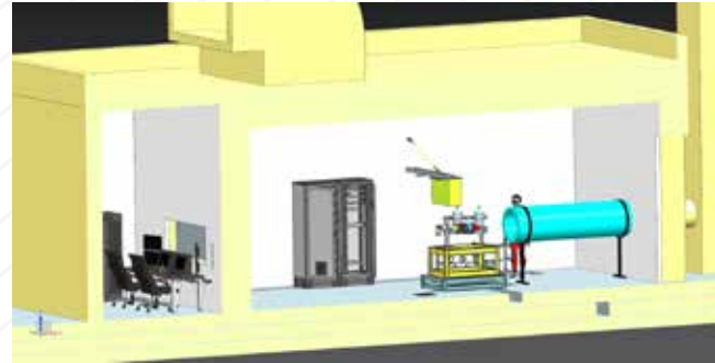
Figure 3. TEI-TJ300 Engine Cell Design
